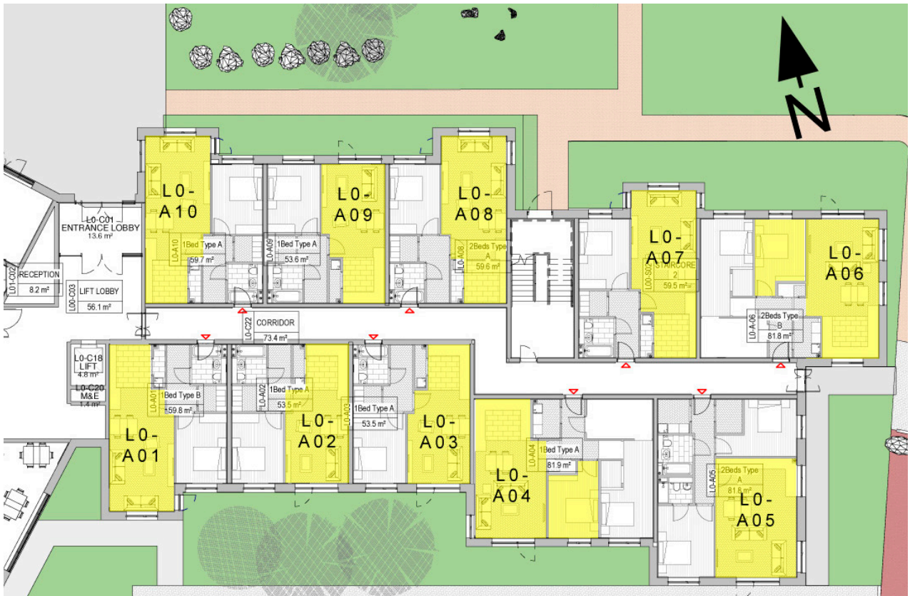
Figure 2: Indicative diagram based on floor plan prepared by Reddy Architecture + Urbanism showing location of sample rooms in the proposed apartment block at the south of the site analysed as part of this assessment of daylight access – annotated in yellow by ARC
