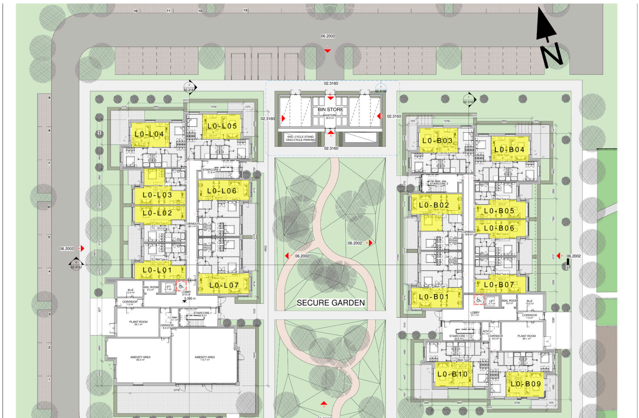
Figure 3: Indicative diagram based on floor plan prepared by ReddyArchitecture + Urbanism showing location of sample rooms in the proposed apartment blocks at the north of the site analysed as part of this assessment of daylight access – annotated in yellow by ARC
